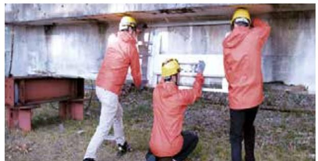
Non-destructive inspection to visualize fractures in steel materials inside a bridge
